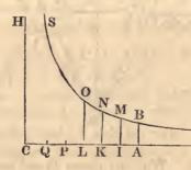
15. PROP. VIII. Let C A represent the force of gravity, A K the resistance,  $\therefore$  C K represents the absolute force at any time (if the body descend); A P, a mean proportional to A C and A K, represents the velocity; K L, P Q are contemporaneous increments of the resistance and the velocity.
